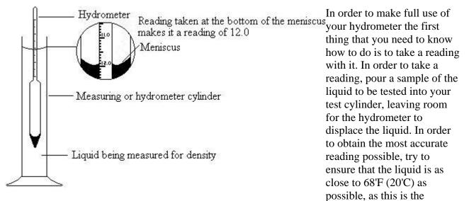
temperature that the hydrometer has been calibrated to (should your hydrometer be calibrated to a different temperature, which should be stated on the meter, ensure that your liquid is at the quoted temperature). Place your hydrometer in the liquid and spin it in order to dislodge any bubbles that may be in the liquid, which would otherwise cause you to get a false high reading. Read the number on the paper where the liquid crosses the stem of the hydrometer.
