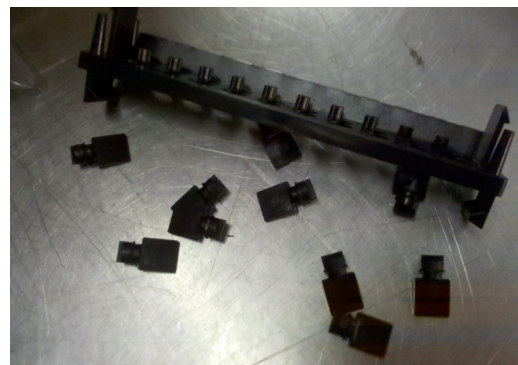
Remove these to access the line ON / OFF adjusting screws on newer manifolds
