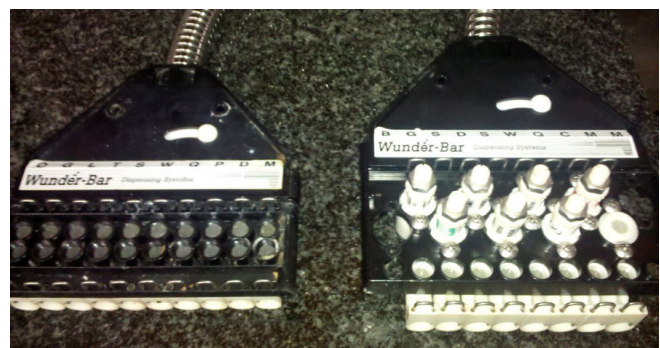
Standard or Low Profile manifold (left) Flow Control or Raised Cone manifold (right)
